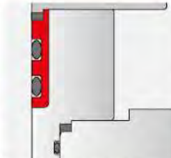
Stem Pocket Welded Overlay 3 mm finished thickness Dynamic seal area.
