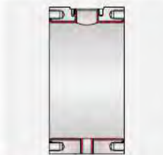
Body Internal Lining On All Wetted Parts min. 300 microns thickness.
