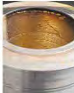
Closure Weld Overlay On All Wetted Parts 3 mm finished thickness.
