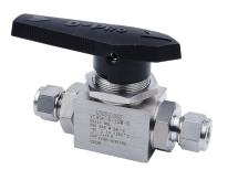
• 2-way On-Off Valves Working Pressure: 274 bar at 120°C • DK-LOK® 3/8" to 1" OD. • Pipe Thread 3/8" to 3/4" Dynamic Seat Design • Orifice: 0.472" (12.0mm)
